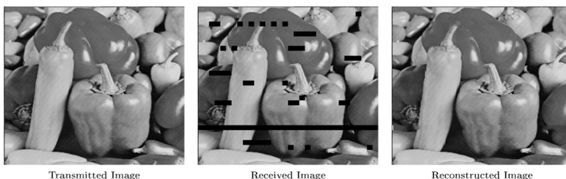
Fig. 4. Restoration result of missed block by [9].
